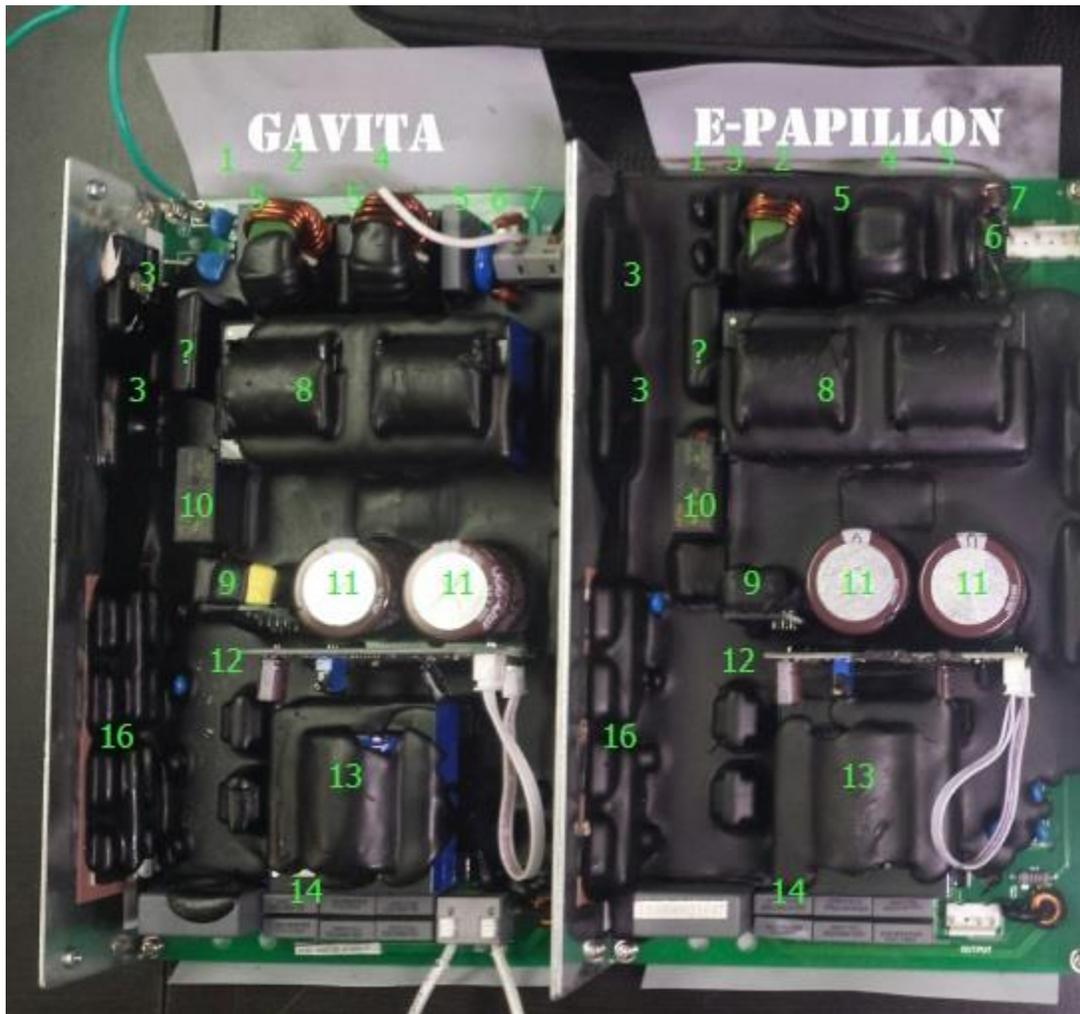
Labels are provided above since it is otherwise nearly impossible to tell them apart. They are twins down to the lengths and placement of the test loops, the choice of semiconductors, brand and size of capacitors, and the direction and placement of passive components. The circuit board even duplicates the shape and placement of the printed wiring traces as can be seen at the bottom of the photo. These are not analogues, these are COPIES. EXACT DUPLICATES. Look at the photo, it's pretty clear.
