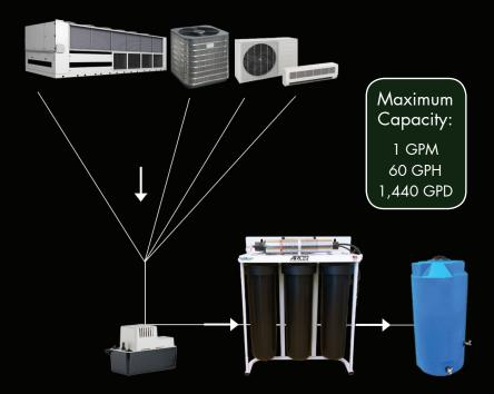
Turn-Key solution includes: Sump pump, 4 stage filter, floor stand and 20' of tubing
